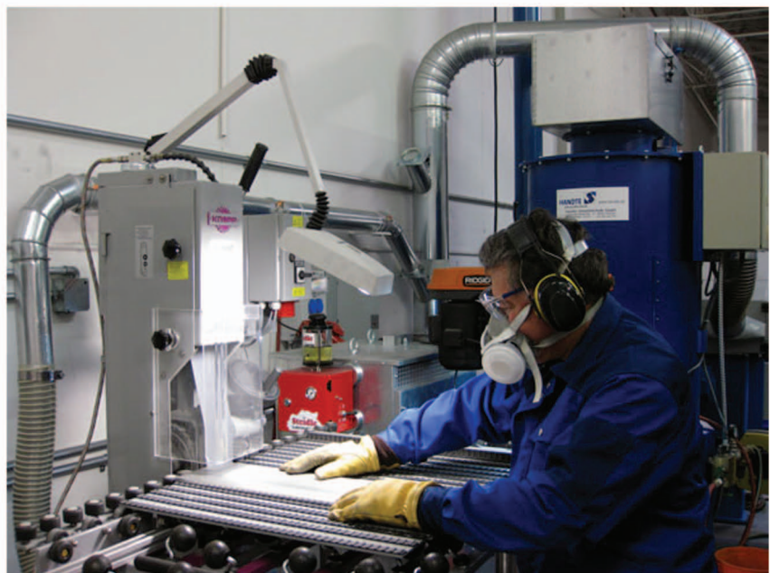
Edges being polished by a master craftsman at the YG Acoustics factory
